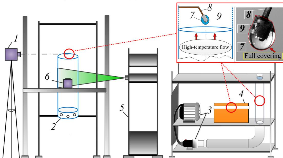
**Figure 1. Scheme of experimental setup: 1 – high-speed camera; 2 – burner with cylindrical channel; 3 – hot air blower; 4 – muffle furnace; 5 – optical diagnostics of combustion products rate; 6 – cross-correlation camera; 7 – liquid droplet; 8 – ceramic rod; 9 – solid inclusion**
